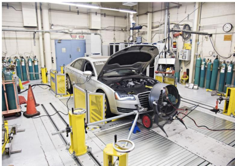
Figure 1: A car is tested on a chassis dynamometer in a lab (Source: Pittsburgh Post-Gazette).
